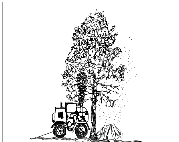
Figure 5 : Keep all construction equipment, generators, and static machinery well away from the branch spread. Do not light any fires or create any source of heat or noxious fumes within the branch spread of a tree.
