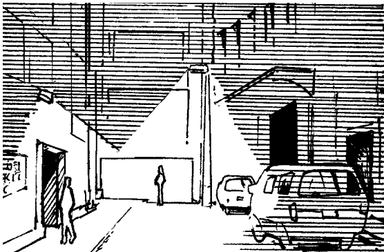
7.2 Lighting on high masts and walls to deter criminal activity
