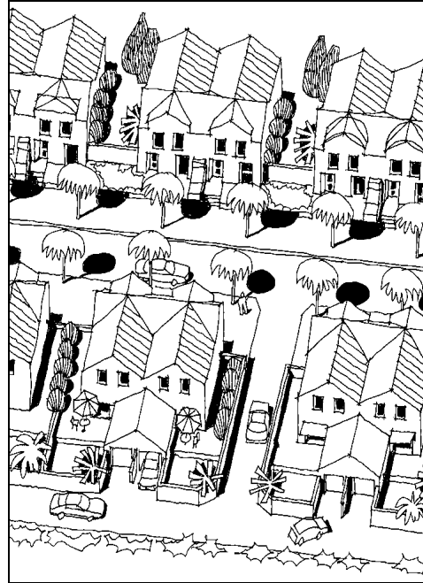
6. Car parking should not dominate the road. An alternative may be to provide access to the rear of properties.
