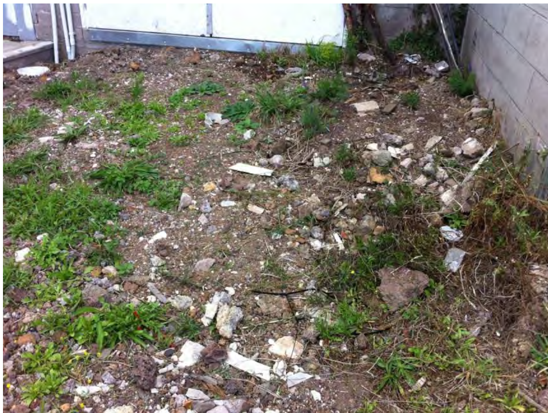
Photograph 21: Suspected ACM fragments from degrading building cladding in southwest part of the commercial area next to the 2 Degrees electrical cabinet.
