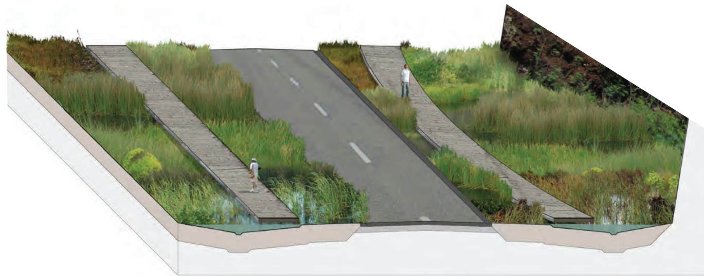
fig. 17: Illustrative section of the wetland roads with native planting, boardwalks, and water treatment ponds lining the roadway
