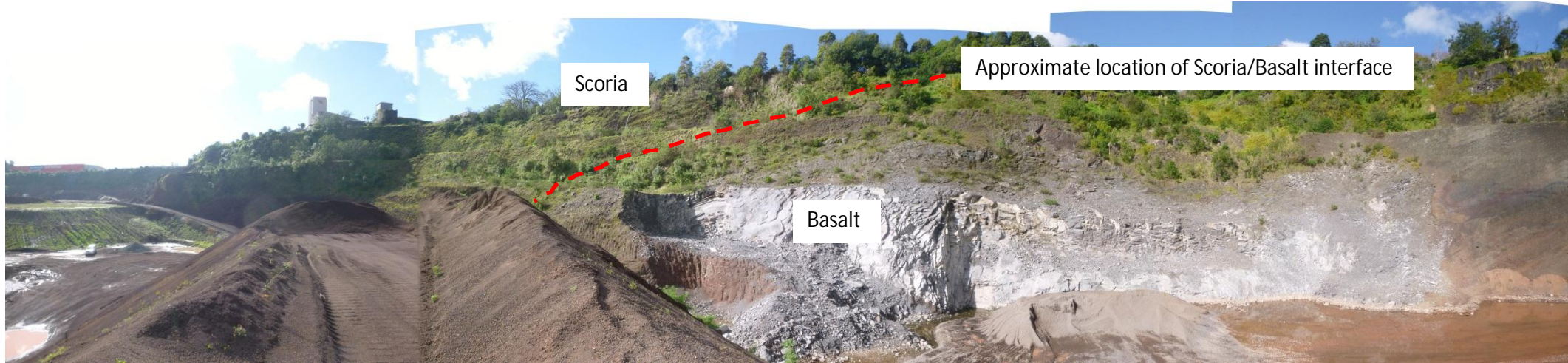
Figure 1: Panorama image of the basalt/scoria quarry face from the south eastern extent of the Three Kings Quarry, Mt Eden. The red dashed line represents the approximate location of the scoria/basalt interface based on field observations.
