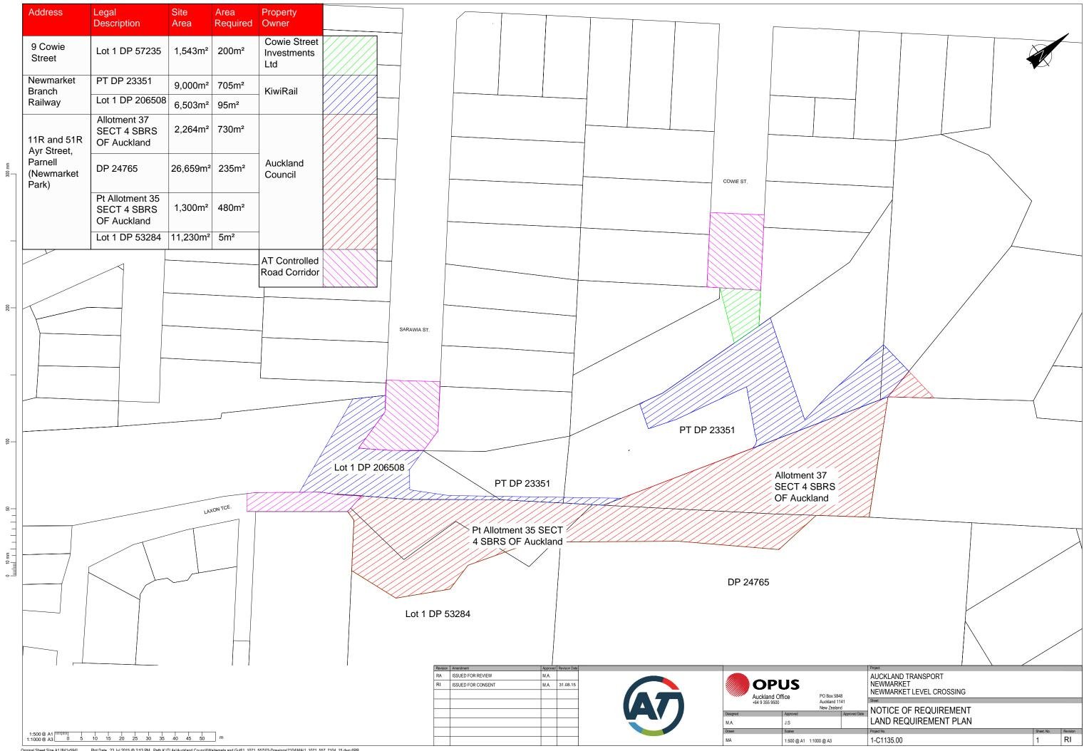
Original Sheet Size A1 [841x594] Plot Date 23 Jul 2015 @ 2.53 PM Path K:\TLAs\Auckland Council\Waitemata and Gulf\\_1071\_557/03-Drawings\7104\MA\1\_1071\_557\_7104\_15.dwg 6RB
