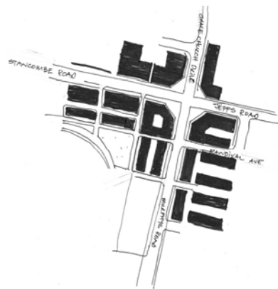
Alternative simple intersection that provides good connectivity and appropriate block sizes, a strong spatial form and does not prioritise one movement.
