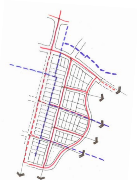
Alternative subdivision pattern which respects the previous lot boundaries and allows incremental development, but allows good connections to occur to future stages with more than one connection to a lot.
