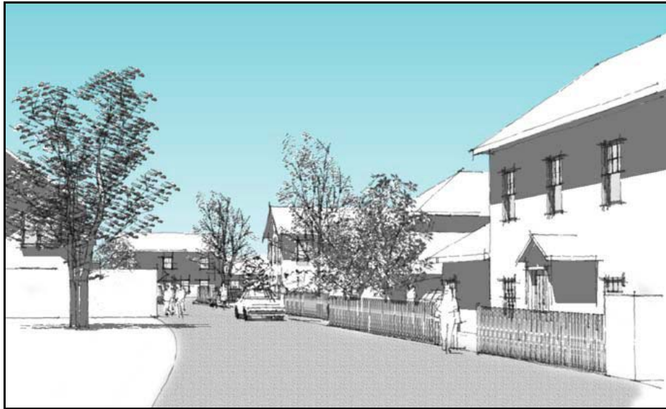
FIGURE 7 Shared surface design with minimal use of defined kerb line, drainage could be accommodated by slot drains and dish channels
