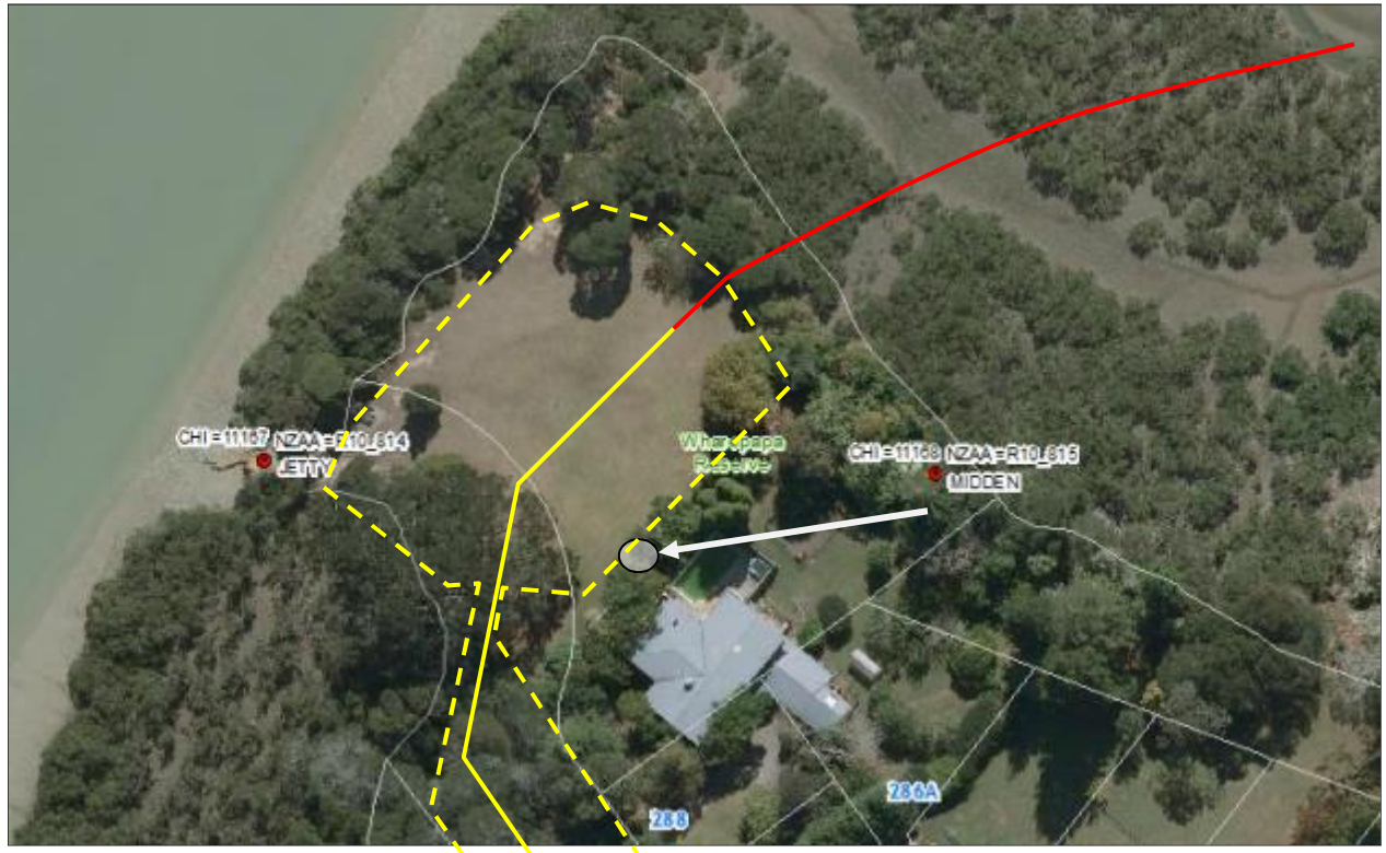
Figure 60. Aerial showing location of sites R10/814 and R10/815 in relation to the proposed designation boundary (dashed yellow line) and the proposed alignment (shown in yellow for open trenching and red for trenchless construction). Aerial source: Auckland Council GIS 2016
