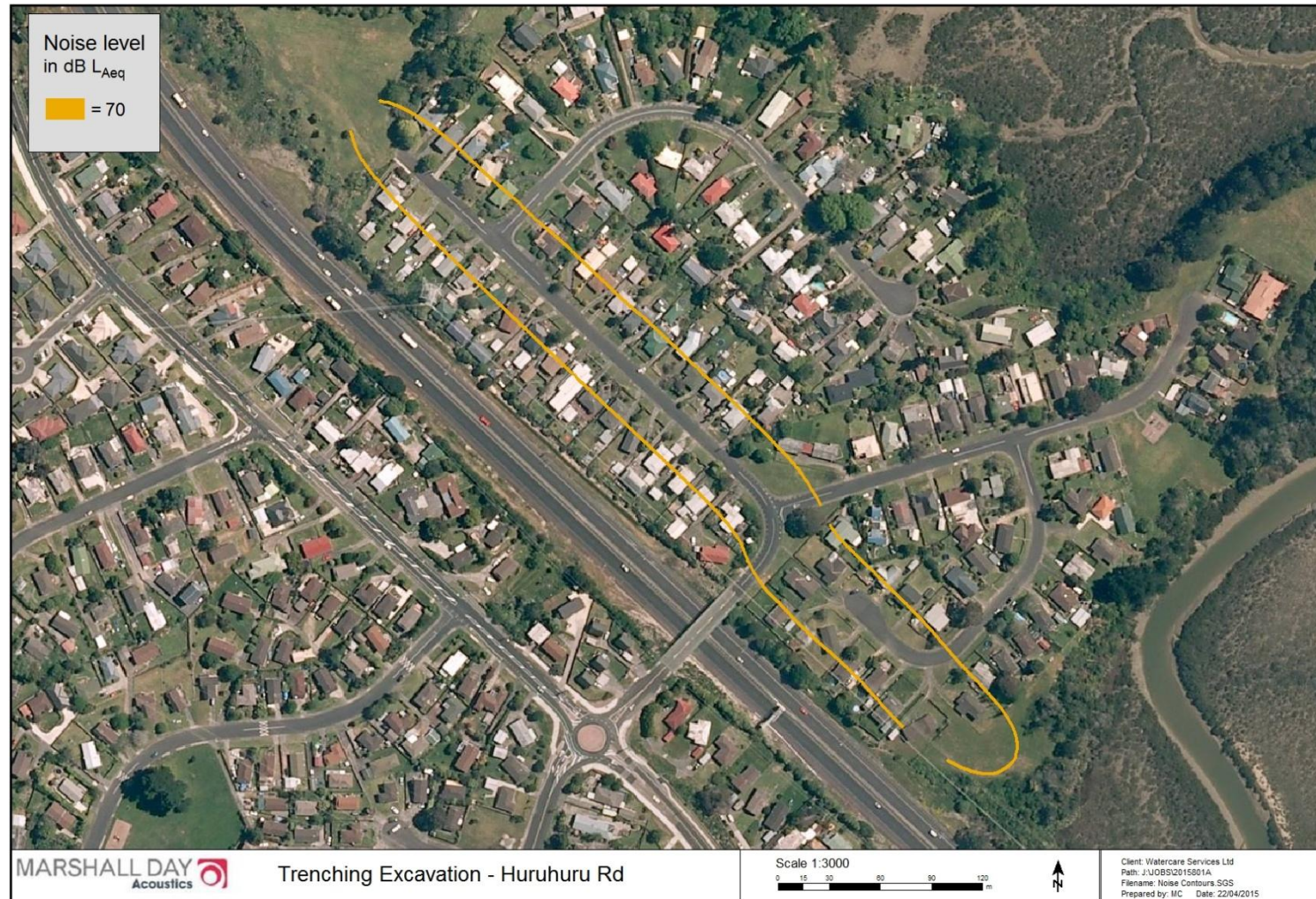
Figure I3: Huruhuru Rd Trenching
