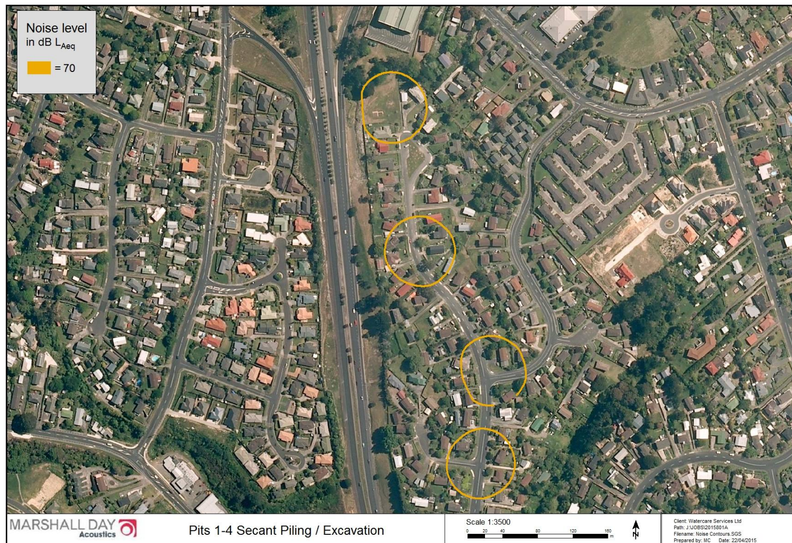
Figure 15: Pits 1 to 4 Secant Piling / Excavation
