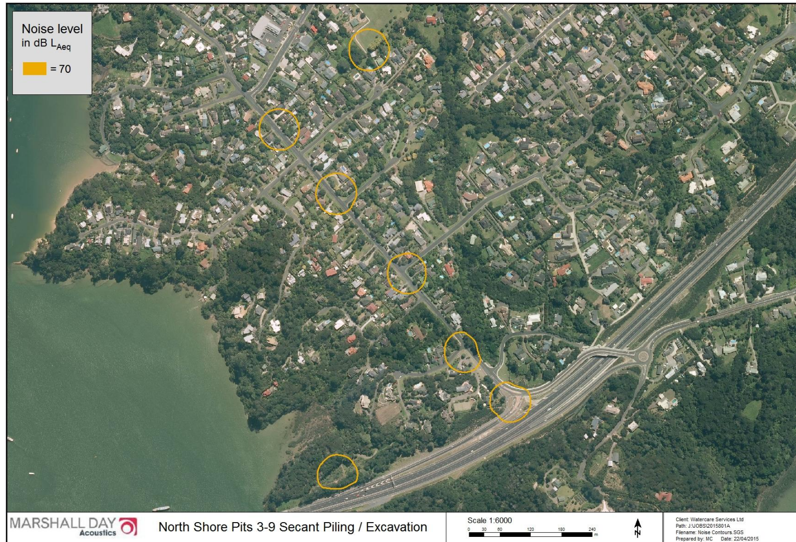
Figure 10: North Shore Pits 3 to 9 Secant Piling / Excavation
