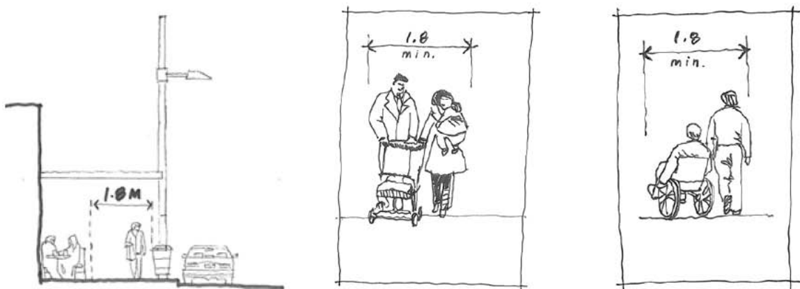
Section and sketches showing minimum 1.8m unobstructed area, allowing for safe comfortable walking/passing of pedestrians, wheelchairs and pushchairs/strollers
