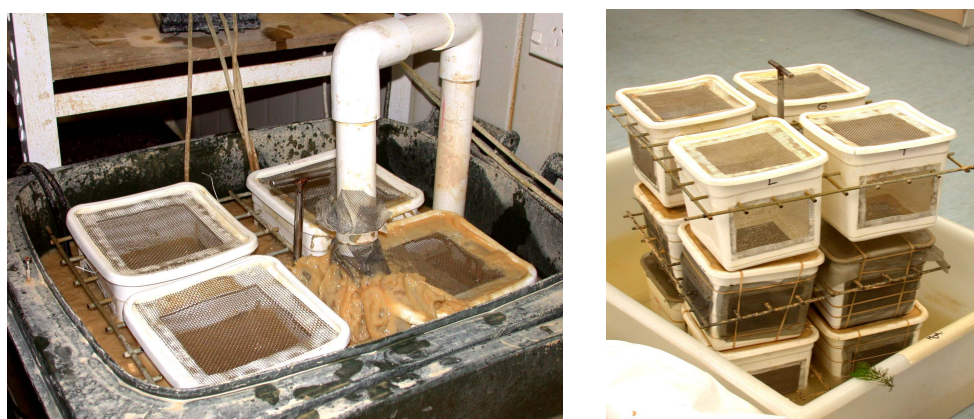
Figure 2. The bin used for maintaining high turbidities and the array of cages housing the animals.
