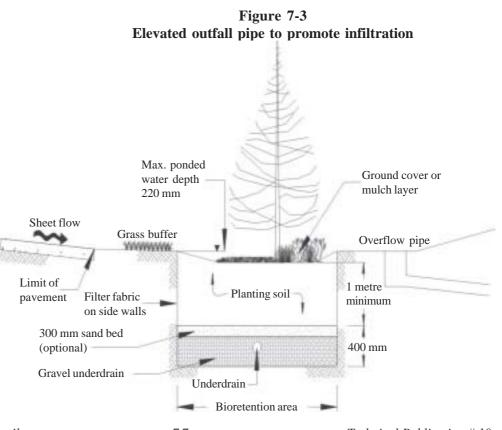
An underdrain must always be used in both designs.
