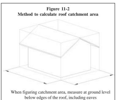
> for proposed buildings this area can be calculated from the architectural plans. Figure 11-2 provides detail on calculating catchment area.
