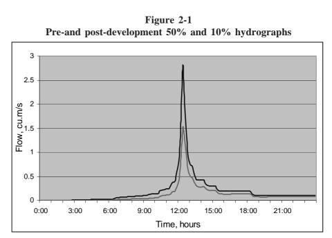
the 50% AEP event increases from 1.51 m<sup>3</sup>/sec to 2.80 m<sup>3</sup>/sec and for the 10% AEP event increases from 2.7 m<sup>3</sup>/s to 4.37 m<sup>3</sup>/s. The volume of stormwater runoff for the 50% AEP event increases from 10,200 m<sup>3</sup> to 16,800 m<sup>3</sup>.
