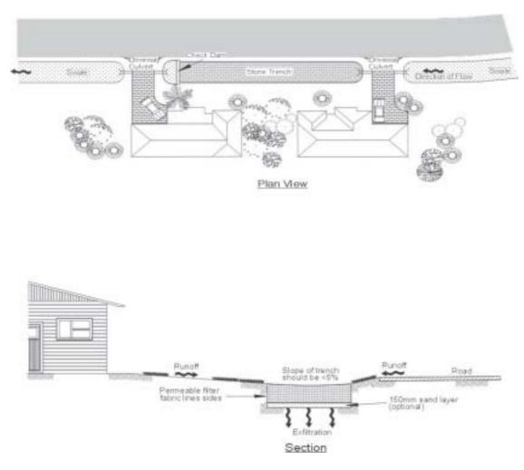
Figure 8-4 Typical detail for an infiltration drywell
