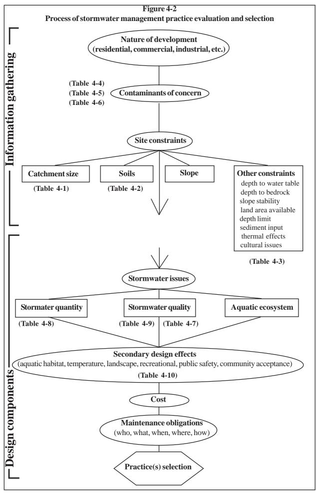
Water quantity practices involve the storage of stormwater and release over a longer period of time to manage downstream flooding. Stream channel stability is not an issue so that the storage and release of the first 34.5 mm of rainfall over a 24 hour period is not an issue. What can be considered is a dry stormwater detention pond whose purpose is to reduce outflow rates to pre-development levels. This does not address water quality, which will need to be considered with a separate practice.
