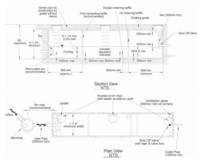
done). Therefore, emphasis must be given to proper application, design, operation and maintenance and prevention of plugging. Other treatment systems, such as sand filters should be considered for the removal of insoluble oil and TPH.
