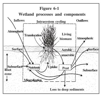
This means that the treatment efficiency achieved by a particular wetland varies widely for different contaminants. In areas with a marked seasonal variation in water temperature, treatment efficiency for a particular contaminant may also vary seasonally.
