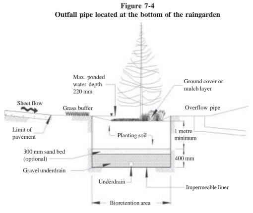
The gravel underdrain will collect and distribute treated excess runoff. A properly designed underdrain system helps keep the soil from becoming saturated. The underdrain system consists of a gravel layer with a 100 - 150 mm perforated piping system. There should be a minimum of 50 mm of gravel cover over the perforated pipe.
