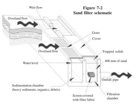
weir in the stormwater channel or pipe. When additional runoff greater than the water quality volume enters the diversion weir area, it will spill over the weir, and mixing with water stored in the filter will be minimal.
