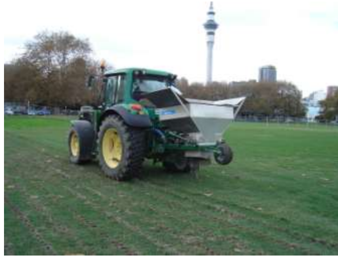
Figure 19 The “gravel banding machine” operating at Victoria Park. The unit has been lifted out of the soil and the expander leg is visible beneath the gravel-containing hopper (after SSDM, 2009).
