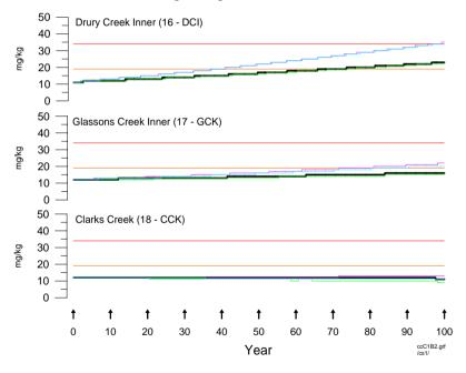
Sensitivity of Scenario 1 predictions to various combinations of doubling the sediment and metal runoff. Year 1 is 2001 and year 100 is 2100. Metal concentration is total metal per total sediment in the surface mixed layer.
