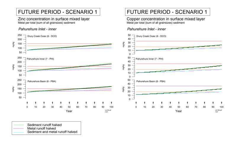
Sensitivity of Scenario 1 predictions to various combinations of halving the sediment and metal runoff. Year 1 is 2001 and year 100 is 2100. Metal concentration is total metal per total sediment in the surface mixed layer.
