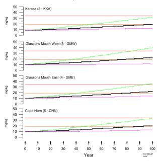
Sensitivity of Scenario 1 predictions to various combinations of halving and doubling the sediment and metal runoff. Year 1 is 2001 and year 100 is 2100. Metal concentration is total metal per total sediment in the surface mixed layer.
