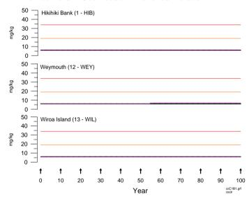
Sensitivity of Scenario 1 predictions to various combinations of halving and doubling the sediment and metal runoff. Year 1 is 2001 and year 100 is 2100. Metal concentration is total metal per total sediment in the surface mixed layer.
