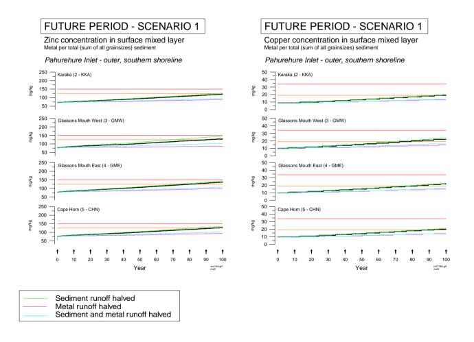
Sensitivity of Scenario 1 predictions to various combinations of halving the sediment and metal runoff. Year 1 is 2001 and year 100 is 2100. Metal concentration is total metal per total sediment in the surface mixed layer.
