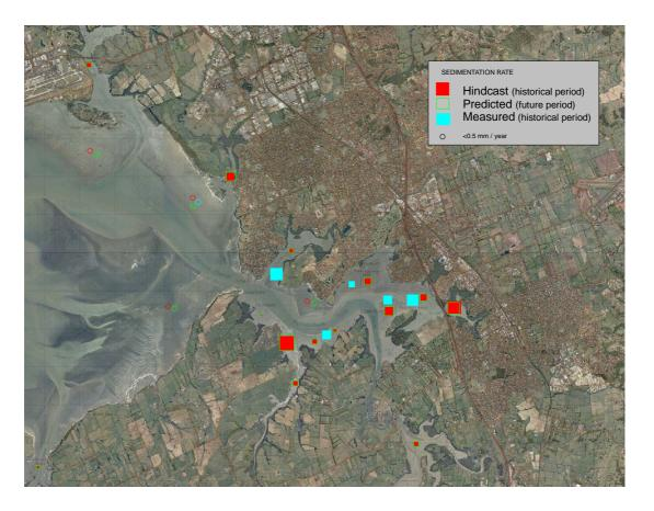
**Figure 4.26:**Predicted change in bed-sediment level over the future period (average of 50 model runs in the Monte Carlo package).
