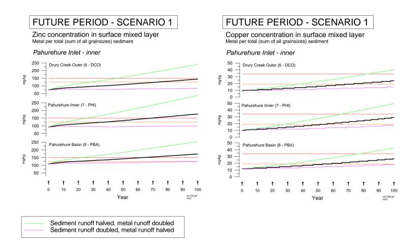
Sensitivity of Scenario 1 predictions to various combinations of halving and doubling the sediment and metal runoff. Year 1 is 2001 and year 100 is 2100. Metal concentration is total metal per total sediment in the surface mixed layer.
