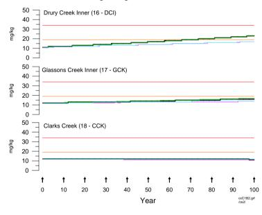
Sensitivity of Scenario 1 predictions to various combinations of halving the sediment and metal runoff. Year 1 is 2001 and year 100 is 2100. Metal concentration is total metal per total sediment in the surface mixed layer.
