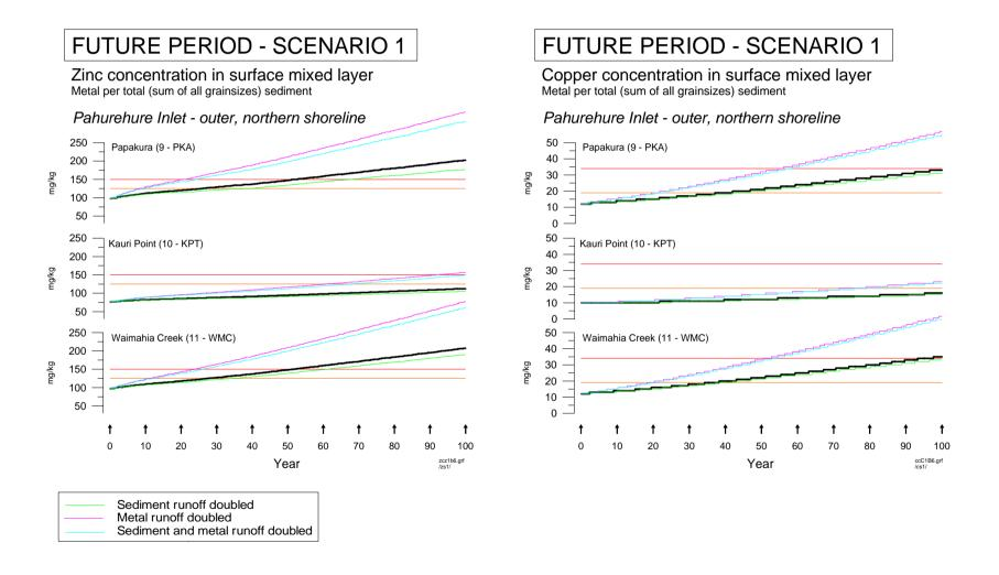
Sensitivity of Scenario 1 predictions to various combinations of halving the sediment and metal runoff. Year 1 is 2001 and year 100 is 2100. Metal concentration is total metal per total sediment in the surface mixed layer.
